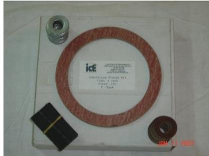
● **Type "E" Gaskets** have the same outside diameter as the flanges, and are made with precision-located bolt holes. They are easy to center and will prevent foreign material from becoming lodged between the flange faces and "shorting out" the flange insulation. Type "E" gaskets are available in any of the materials described on this data sheet.
